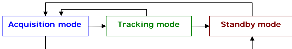
Figure 23: Operational Flow of the AIRES earth sensor.
